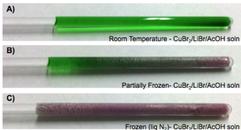
Figure 4.12. The 5 mM \text{CuBr}_2 /100 mM LiBr solution in AcOH shows thermochromic behavior. It is (A) emerald green at room temperature and (B, C) purple when frozen (77 or 145 K).
