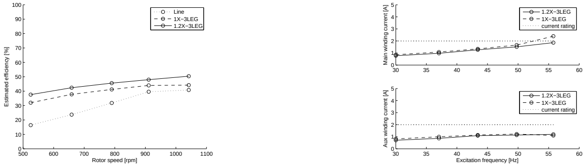
Figure 8.12 Comparison of motor estimated efficiency under line operation, 1X-3LEG inverter operation, and 1.2X-3LEG inverter operation. This plot can be compared to Figure 7.3.
