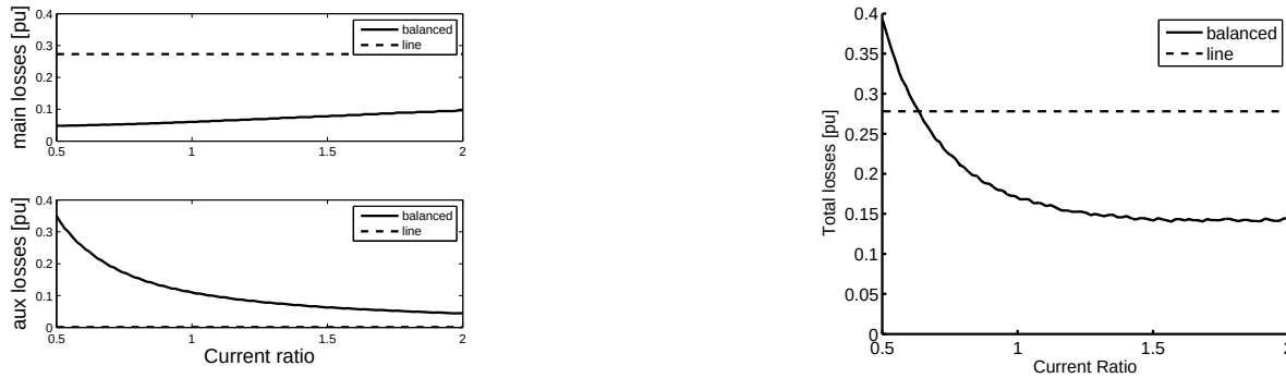
Figure 7.4 Power loss a) in each stator winding and b) both the windings as a function of mmf ratio
