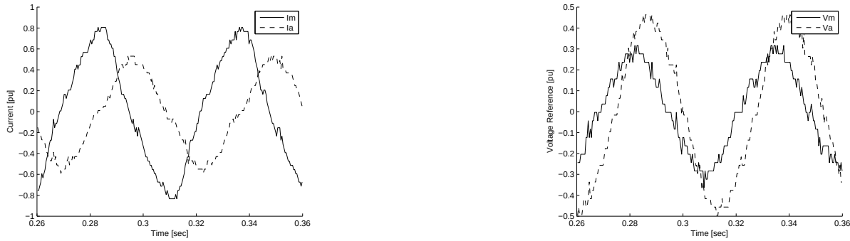
Figure 8.4 Voltage and current waveforms at an output frequency of 20 Hz. Under constant V/Hz, the output voltage is 0.3. The noise in the waveforms is primarily due to DAC output limits and oscilloscope quantization.
