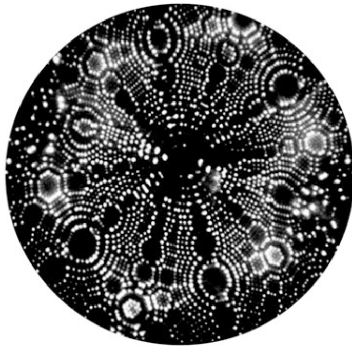
Figure 2.10: Field ion image of \langle 110 \rangle zone axis of tungsten. Reproduced from [65].
