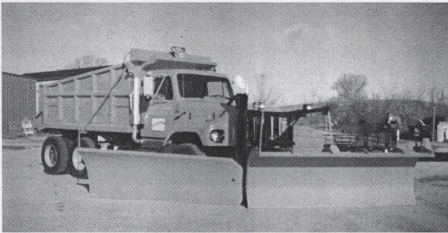
1993 tandem axle dump truck with plow and wing attachment. Town of Menasha.
