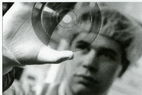
A Blu-Ray disc researcher inspecting a manufactured BD-ROM disc for errors.
