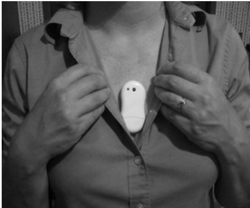
Figure 10-1: Commercialized Hot Flash monitor. Placement of the monitor is usually done vertically over the sternum but it can be placed on either side.
