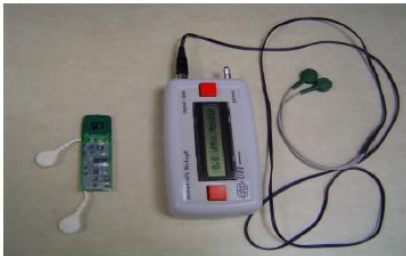
Figure 2: Miniature monitor compared to commercially available Biolog Hot Flash Monitor
