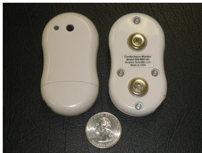
Fig. 9: The size of the monitor is 7.2 cm × 3.8 cm × 1.2 cm and it has a mass of 16 g - 0.56 oz including the battery. The battery has a life of more than 1 week. The conductance range is 0 to 30 \mu S
