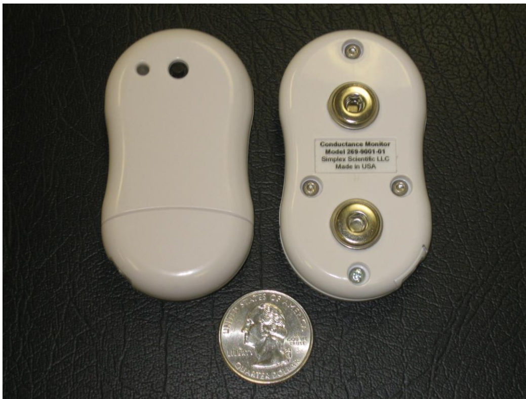
Figure 4-3: The size of the monitor is 7.2 cm × 3.8 cm × 1.2 cm and it has a mass of 16 g or a weight of 0.56 oz including the battery. The battery has a useful life of more than 1 week. The conductance range is from 0 to 30 \mu S.
