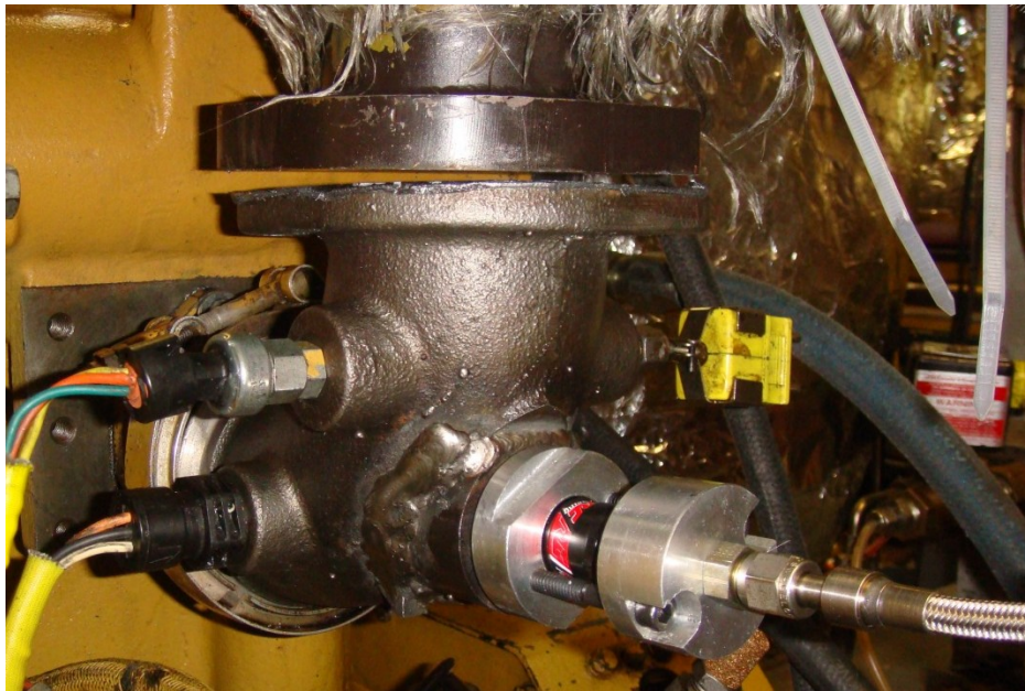
Figure 37 installed port injector in intake elbow
