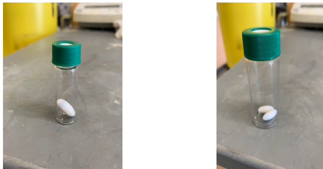
Figure 2A.1. A 1 dram vial for 0.2 mmol reaction with small stir bar (left), and a 24 mL vial for 0.5 and 1.2 mmol reaction with two stir bars (right).
