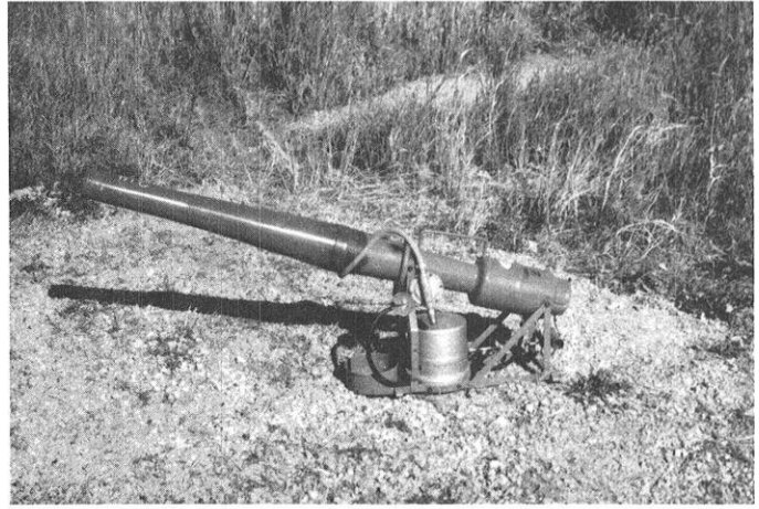
Propane exploders, or "gas cannons" such as this one, are a common tool used in goose damage abatement. They were widely used as a source of disturbance to relocate geese on Horicon National Wildlife Refuge beginning in 1977.
