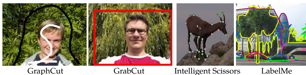
Figure 2.3: State-of-the-art of interactive segmentation methods: Graphcut (Boykov and Jolly, 2001a) and Grabcut (Rother et al., 2004) are region based; (Mortensen and Barrett, 1998) and LabelMe (Russell et al., 2008) are edge based.
