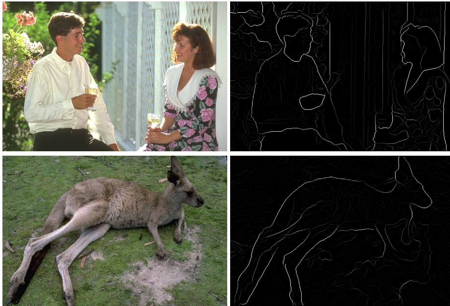
Figure 2.2: Examples of boundary detection using the globalPb contour detector (Arbelaez et al., 2011).
