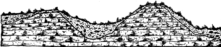
FIG. 33.—Diagrammatic section showing relation of drift to underlying rock where the drift is thin relative to the relief of the underlying rock.
