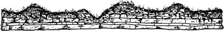
FIG. 47.—Section in a driftless area, showing relation of the mantle rock to the solid rock beneath.
