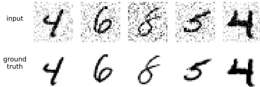
Figure 2.4: The input and ground truth for the image denoising problem. There are 70,000 images in the output, the original MNIST dataset. For the input, random noise is added to images, and amount of data grows to 350,000 input/output images. Each partial_fit calls sees (about) 20,780 examples and each call to score uses 66,500 examples for validation.
