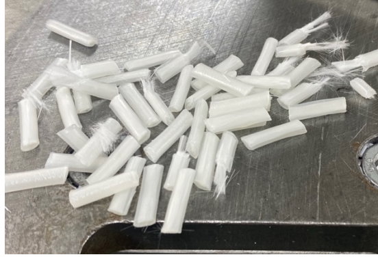
Figure 5.1: Broken pellets found at the bottom of the hopper during the screw pull-out experiment.
