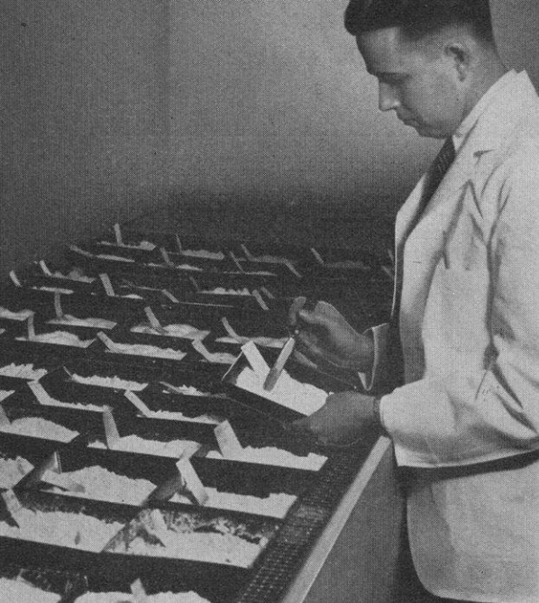
Iodized salt and limestone samples are analyzed to determine effectiveness of various stabilizer levels
