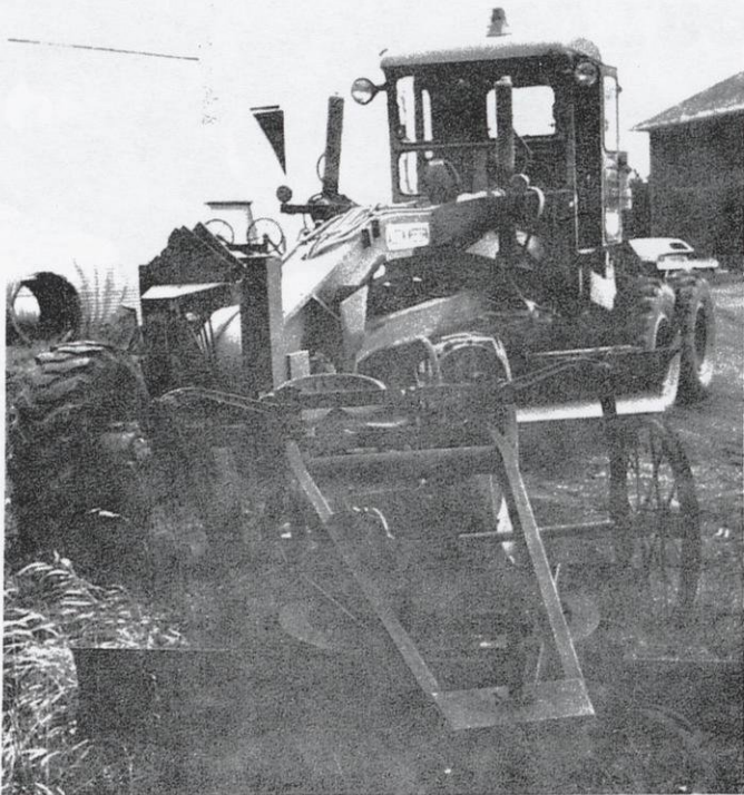
Comparing the old with the new. In front of the Austin-Western grader now used for patrolling the roads of the town, stands an old tractor grader.
