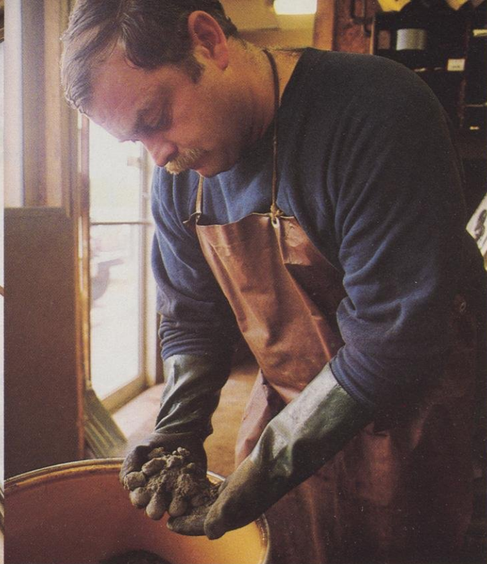
Stouffer precipitates welding residues and metal sludges washed from old radiators. Clean water is decanted off and the pasty mix is dried to a powdery residue that is compact and valuable to a recycler.
