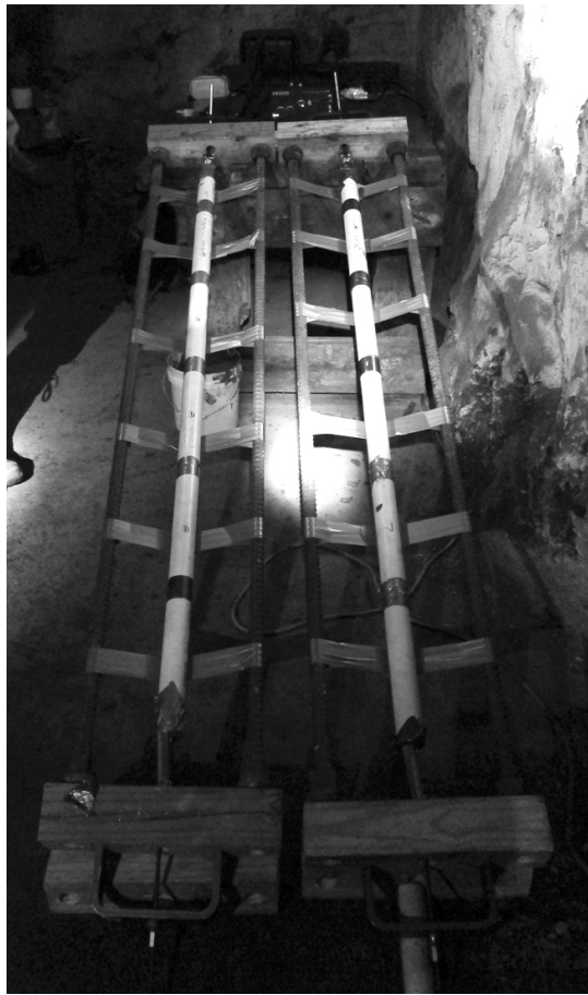
Figure 3.5. Photograph of two FROSTS in pretensioning frames. The FROSTS are grouted into the PVC pipes while being held in tension. The frames are inclined off the table to allow the grout to fully fill the pipe, surrounding the FROSTS, from bottom to top. The duct tape on the PVC pipe covers the breather holes, and the duct tape spanning the rebar provides support for the PVC pipe filled with grout.
