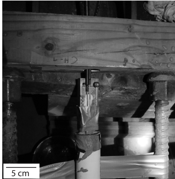
Figure 3.6. Close-up photograph of bracket holding FROSTS in the pretensioning frame.
