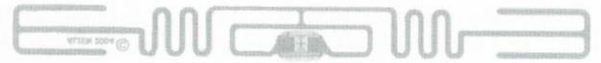
One example of an RFID tag that uses a microchip and a copper antenna on a plastic band.
