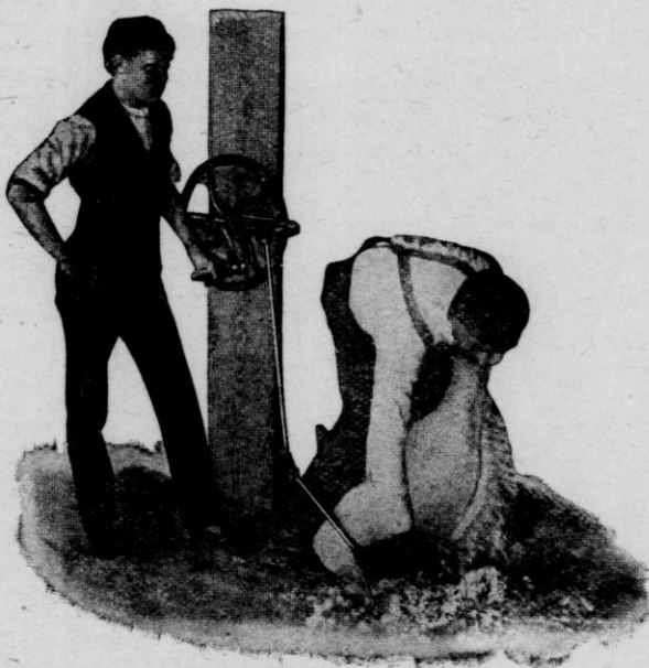
THE CHICAGO FLEXIBLE SHAFT SHEEP SHEARING HAND POWER MACHINE AT WORK.
