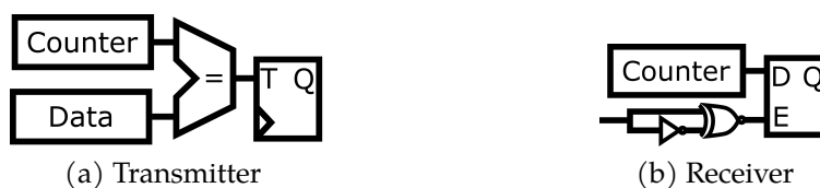
Figure 6.1: Basic Temporal Transmitter and Receiver Designs.
