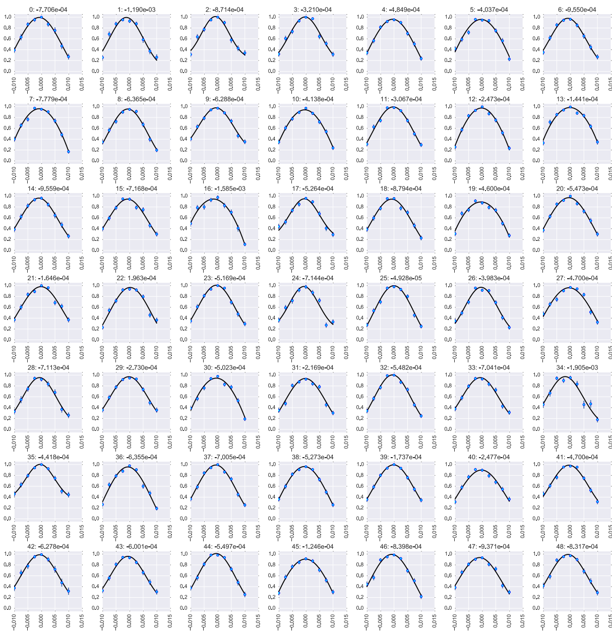
Figure 13.3: Microwave spectroscopy globally on all sites at the same time. Frequency is expressed as MHz change from resonance. Number above each site is the fitted frequency shift in MHz relative to the previous tuning point. Array averaged -5.8(4) \times 10^{-4} MHz. Data from 2015-04-23-08-00-03 and 2015-04-23-08-38-48.
