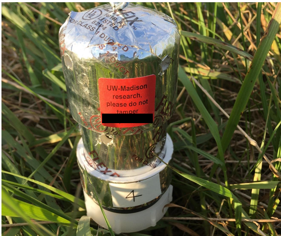
Figure S7. A reflective-foil coated PVC iButton capsule deployed at a 5-cm height in a grassland study site in southern Wisconsin, USA, 2021.
