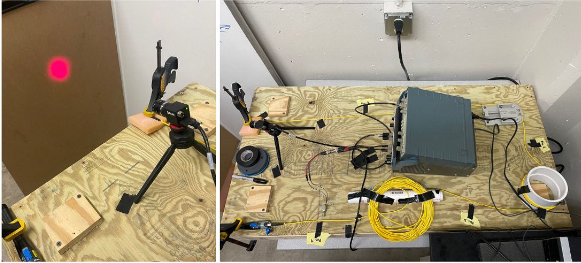
Figure 5.2: Initial experiment of visible light analysis through fiber. Left frame shows projection of visible light, right frame shows setup from light source through 10 m cable on evaluation board.
