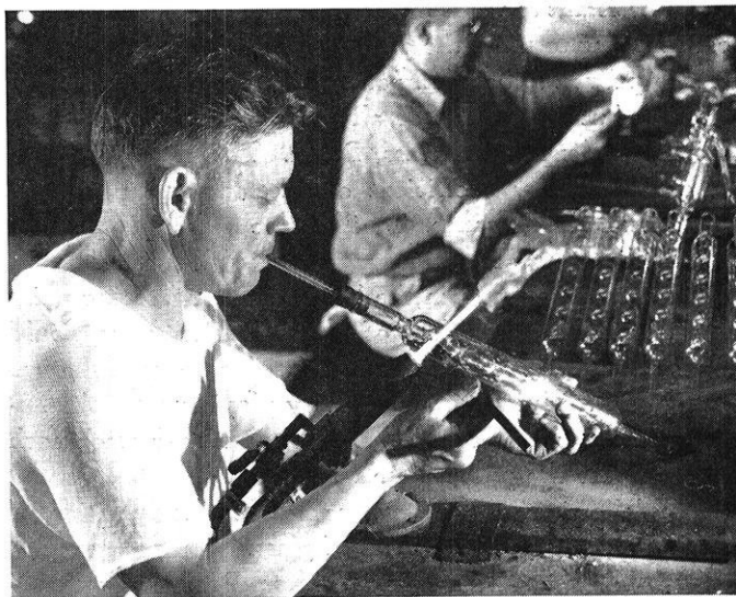
Lamp worker fabricating bulb type condenser.
