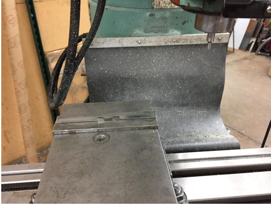
Figure 28 – Tensile sample clamped in the mill, with the edge-finder in the mill chuck
