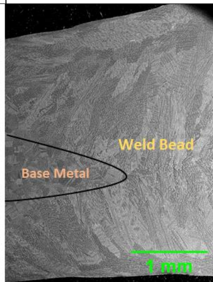
Figure 32 – SEM image of etched 740H weld interface after new weld procedure
