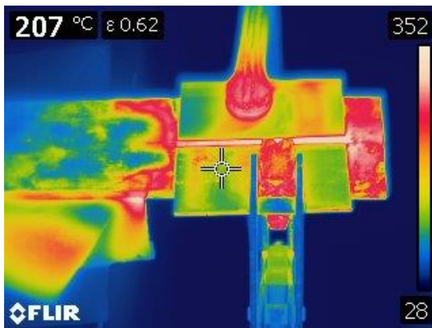
Figure 24 - Thermal image of P92 plates prior to similar welding ( >200^{\circ}\text{C} ), clamped on a copper backing plate
