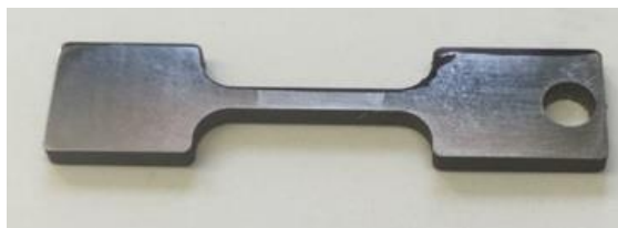
Figure 30 – 740H welded tensile sample etched with glyceric acid showing the weld in the center of the gauge
