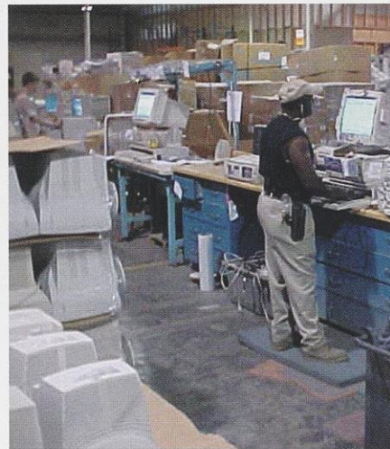
Electronic products like computers are disassembled and "demanufactured" to recover circuit boards, motors, metals and other components. "We view ourselves as 'end of life' processors for electronics," says Karen Birkenstock, executive vice president with 5R Processors, Ltd. that operates three receiving centers in northwest Wisconsin.
