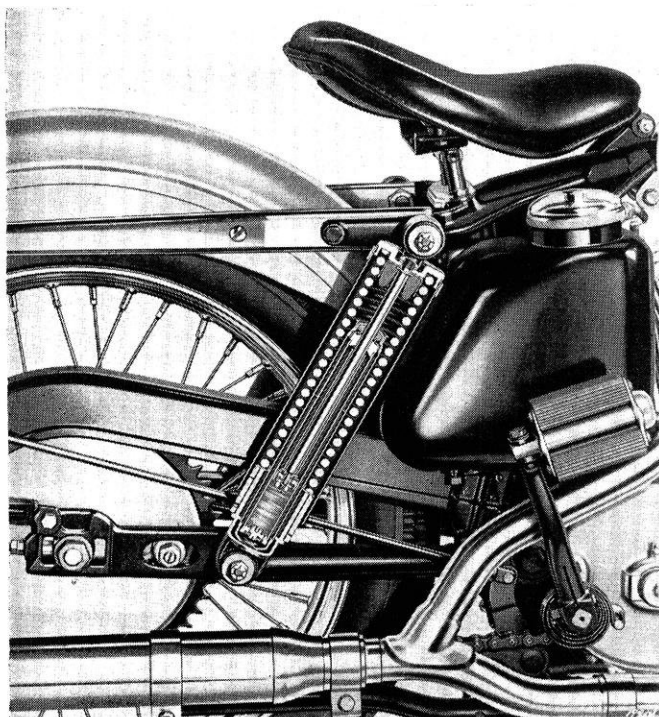
This cutaway shows the swinging arms which position the rear wheel and the coil springs and concentric tubular shock absorbers which limit rear wheel travel.
