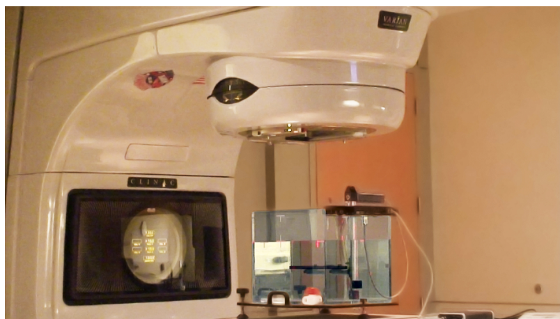
Figure 4.3: Ionization chamber dose measurements of irradiated by the Varian Linac in TG-51 reference conditions
