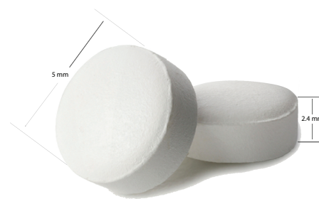
Figure 2.13: L- \alpha -alanine radiation dosimeters
