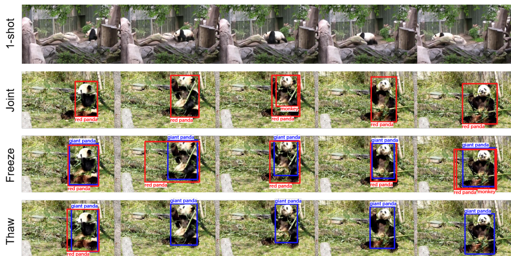
Figure 5.4: Examples of few-shot learning for video object detection of giant panda (weak base dataset). Blue ( resp. red) bounding boxes denote correct ( resp. incorrect) detection. Note that red panda is a different animal. The 1st row shows the 1-shot novel-class video used in few-shot adaptation. The 2nd, 3rd, and 4th rows show the detection results in the validation videos by Joint, Freeze and Thaw, respectively.
