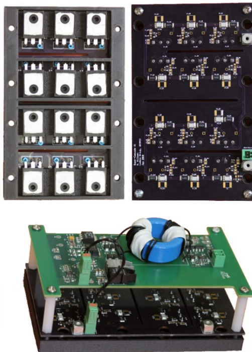
Figure 2-6. Top) Assembled Super-Cascode with mounting bracket, back and front views. Bottom) Super-Cascode with accompanying gate driver
