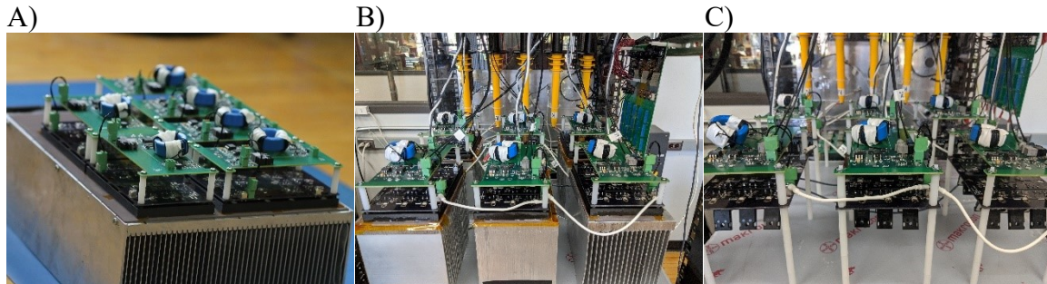
Figure 5-4. Evolution of Super Cascode A) Single Heatsink B) Individual Heatsinks C) No Heatsinks
