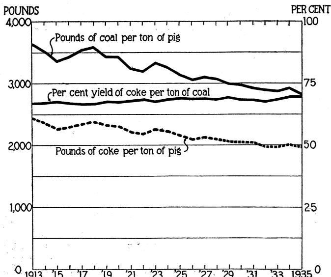
FIGURE 93.—Declining consumption of blast-furnace coke per gross ton of pig iron, 1913–35. The quantity of coke consumed per ton of pig iron has been declining. At the same time, the yield of coke per ton of coal carbonized has increased slightly, so that the consumption of coking coal per ton of pig iron produced has declined from 3,637 pounds in 1913 to 2,838 pounds in 1935.
