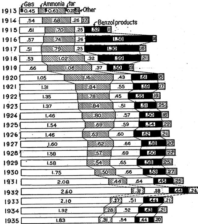
FIGURE 95.—Gross value of the several byproducts per ton of byproduct coke produced, 1913-35.
