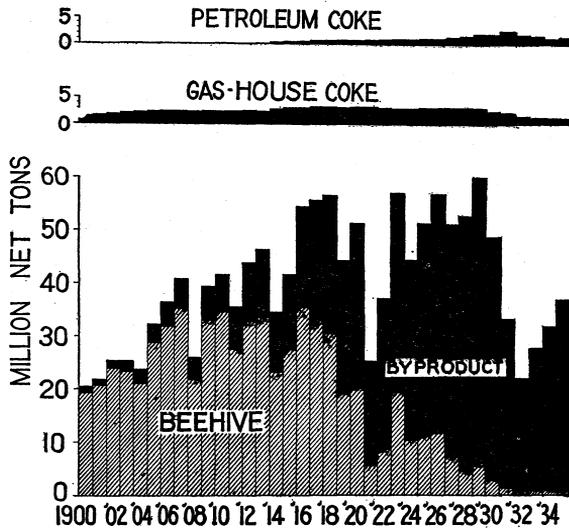
FIGURE 91.—Production of petroleum coke, gas-house coke, and beehive and byproduct coke in the United States, 1900-1935. No figures on production of petroleum coke are available before 1914, when the production was 213,777 tons.
