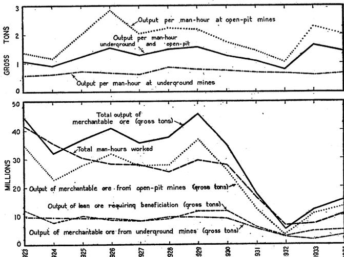
FIGURE 66.—Trends in output of merchantable iron ore per man-hour at open-pit and underground mines in Minnesota compared with production of merchantable and lean ore and total man-hours worked, 1923-34.
