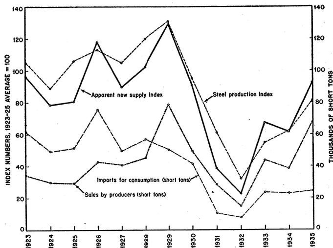
FIGURE 152.—Trends in sales by producers, imports for consumption, and apparent new supply of dead-burned magnesite compared with Federal Reserve Board index of production of steel ingots and castings in the United States, 1923-35.
