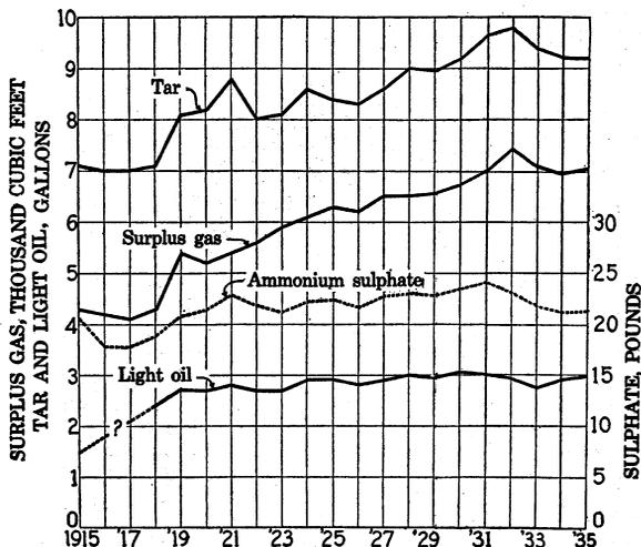
FIGURE 96.—Average yield of principal byproducts per net ton of coal carbonized in byproduct coke ovens, 1915-35. Figures for light oil represent average at plants recovering light oil.
