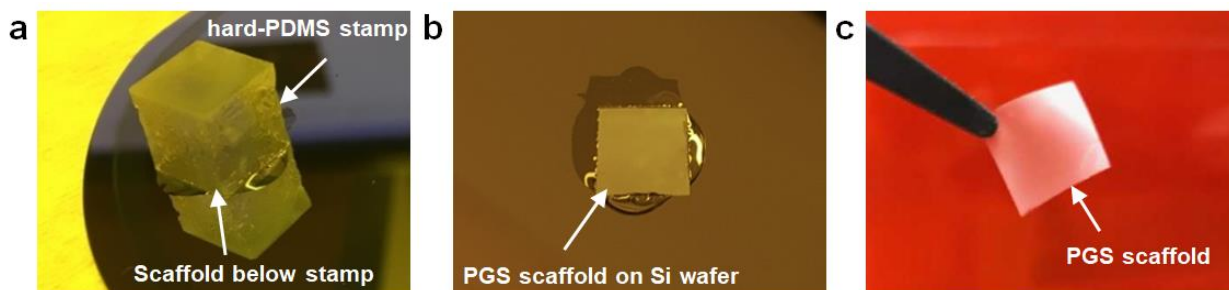
Figure 2.9. Low magnification photographic images depicting the fabrication process of the PGS ice cube tray PR scaffold. a) h-PDMS stamp ready to be demounted from the scaffold on a Si wafer after complete PGS curing. b) A PGS scaffold on the Si wafer after stamp removal. After removing scaffold edges, the scaffold was delaminated from the Si wafer using a single edge razor blade. c) Fabricated PGS ice cube tray scaffold held with fine forceps.
