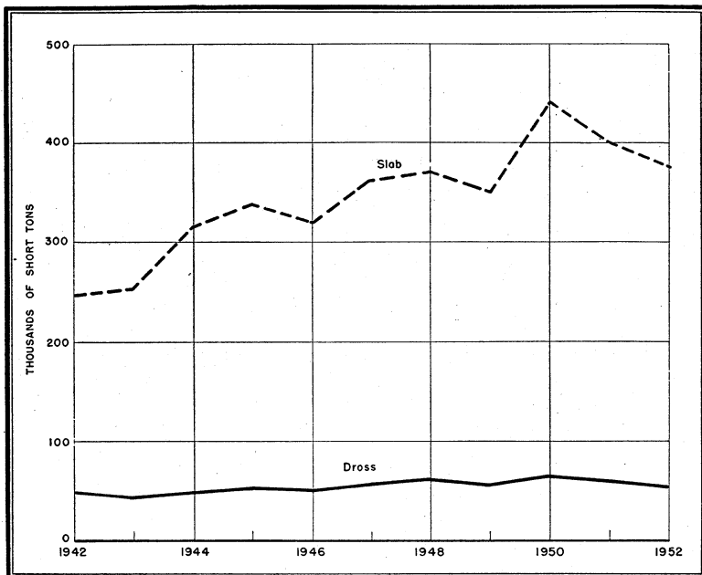
FIGURE 1.—Consumption of slab zinc in galvanizing and of galvanizers' dross, 1942-52.
