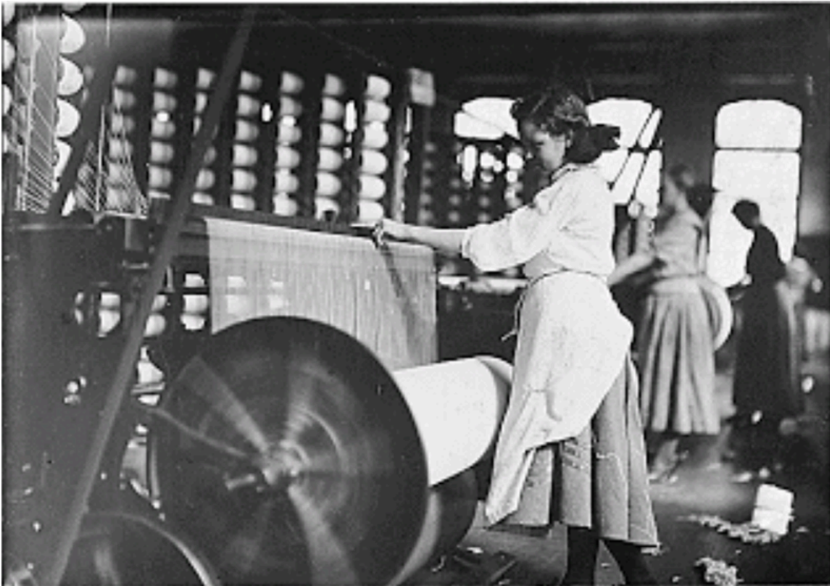
Figure 12: An operative monitoring threads being fed onto a warping beam. As noted, this basic technology for cotton mill production did not radically change between 1850 and 1908 when this image was taken. Lincoln Cotton Mills: Evensville, Ind National Archives and Records Administration ID 523100, image posted on Wikimedia Commons.
