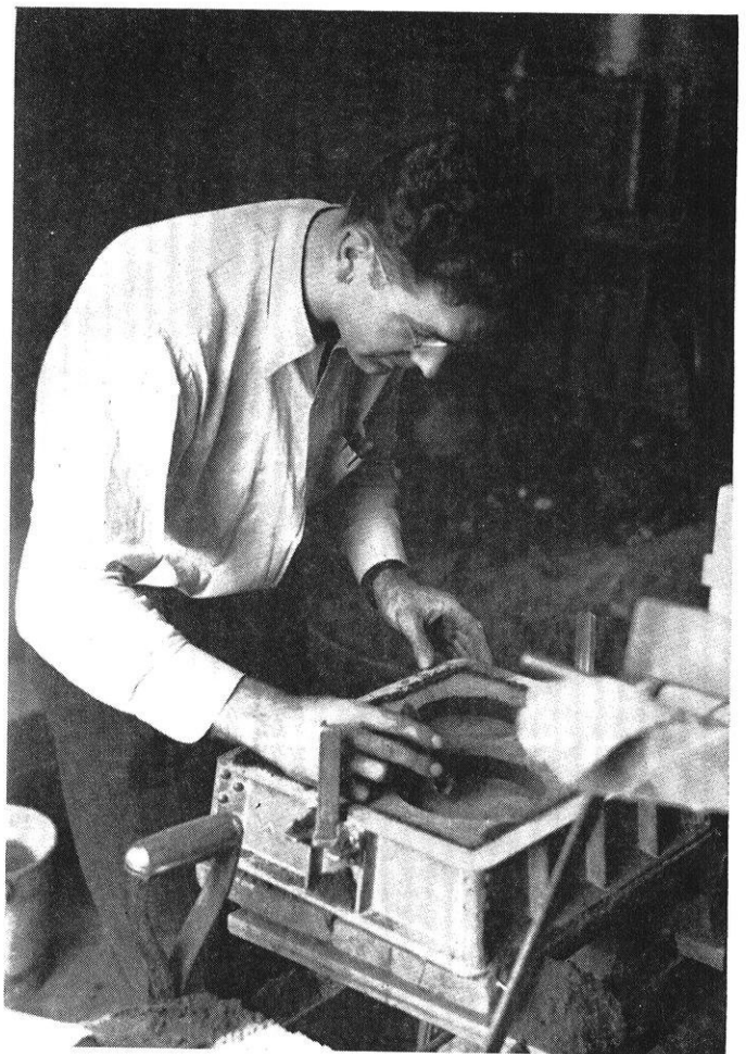
Putting the last touches on the mold in foundry lab.
