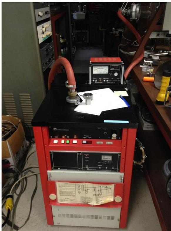
**Figure B.4.** The Leybold-Heraeus Helium leak detector.
