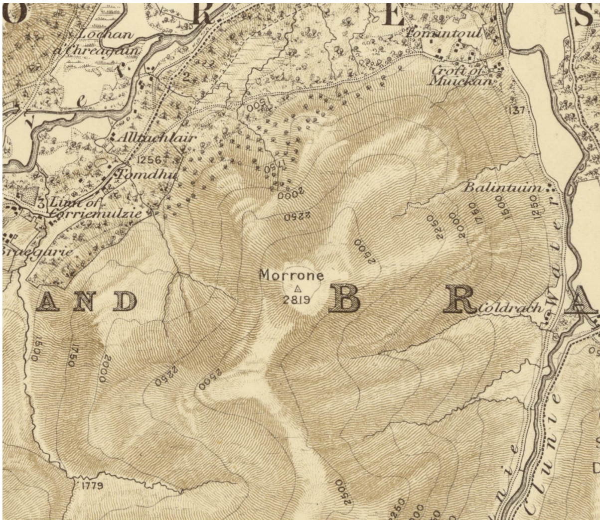
Figure 6.8 Balmoral. Sheet 65. Ordnance Survey of Scotland. 1/M 2E map.1900. 58x71cm. Hachures in brown. Contours in black. Scan by National Library of Scotland.
