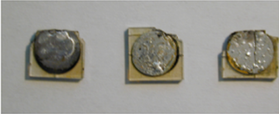
Figure 2.7: Several failed optical switches consisting of 1 cm x 1 cm SiC layers with 1 mm thickness. Failure occurred at an average field strength of 30 MV/m; field enhancement effects at the edges of the electrodes pushed the field strength to approximately 350 MV/m, causing their failure. Image from Caporaso, 2009 [6].
