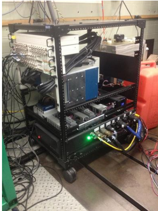
Figure 3.4 Photograph of the Drivven control system
