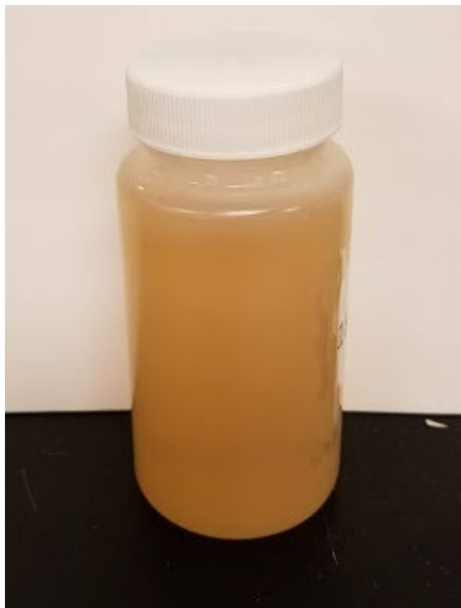
Figure 13. Private Well Sample Collected from Iron County with Iron Concentration of 24.9 mg/L.
