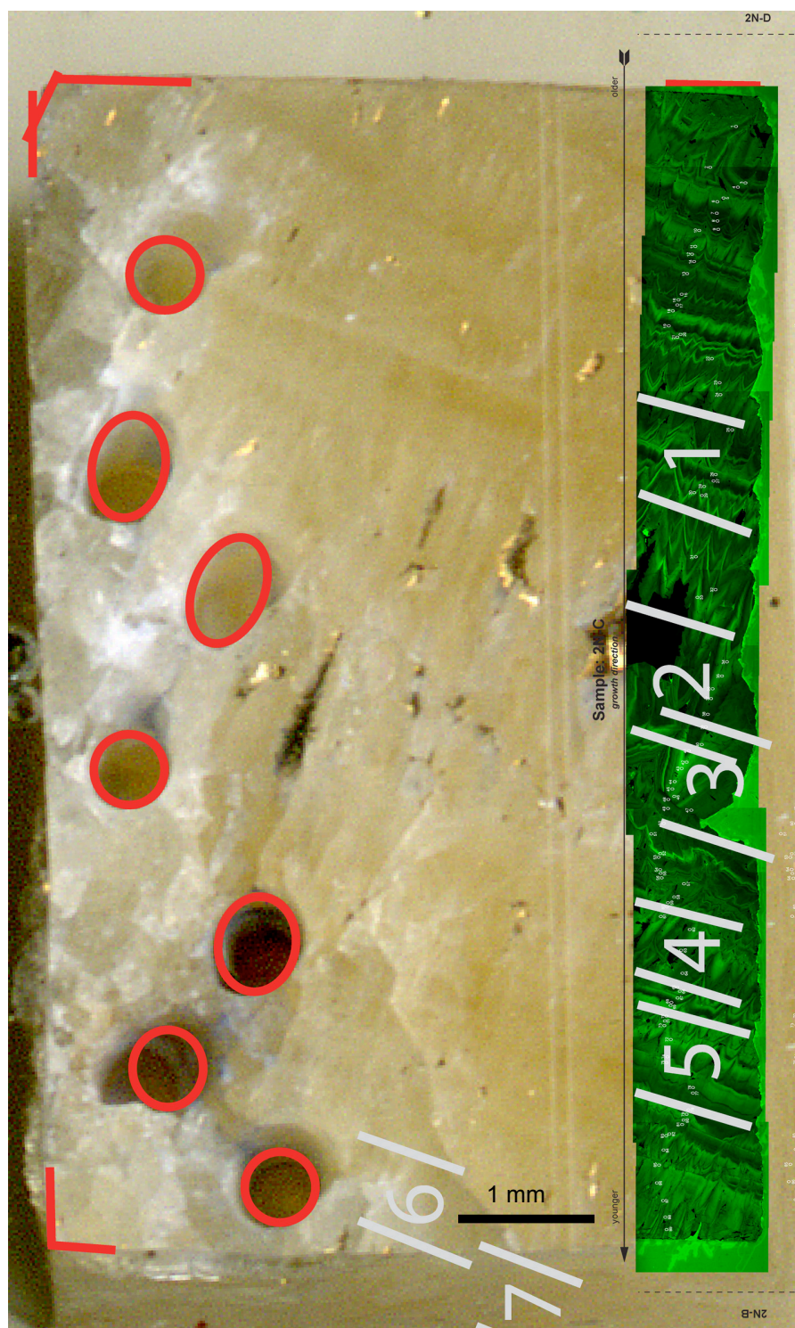
Figure E.3: Projection of the spots in chip 2N-C drilled for acid-digestion \delta^{18}\text{O} analysis (red circles) onto the ion microprobe analytical traverse (composite CLFM image). The gray bars on the ion microprobe traverse (composite CLFM image) indicate the range of calcite sampled by each drill-spot. Table E.6 lists the ion microprobe analyses that each drill spot overlaps.
