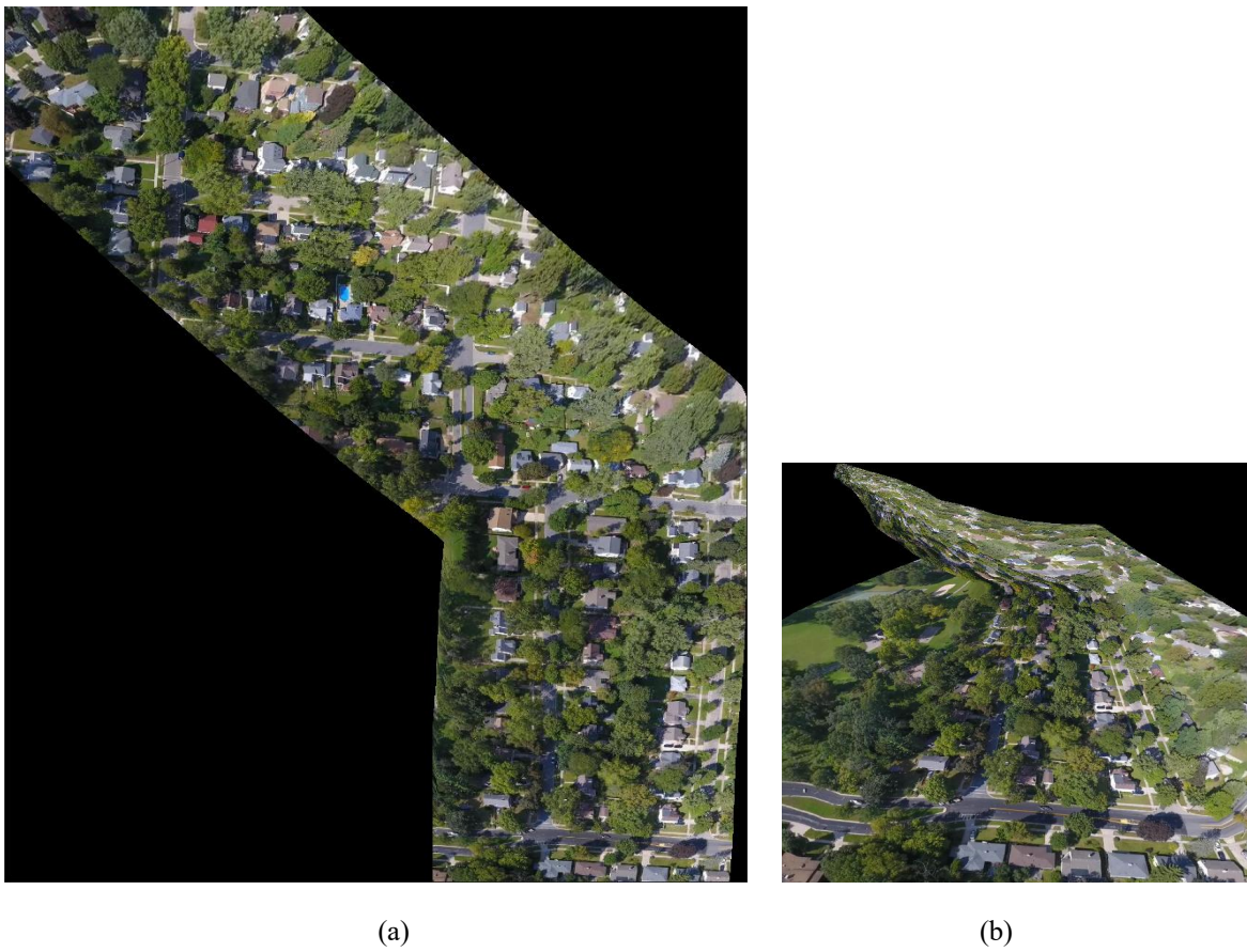
Figure 4.13: Video mosaic result of perspective video with slant flight path using (a) MoB with P2Prectify (b) FB.
