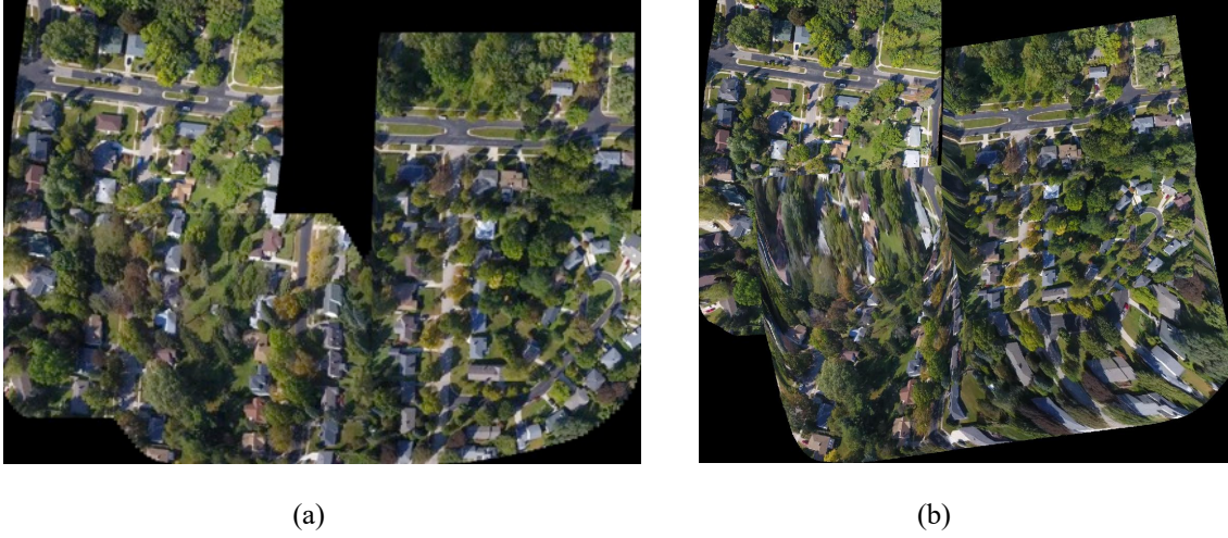
Figure 4.12: Video mosaic result of video with camera angle change mid-flight using (a) MoB with P2Prectify (b) FB.
