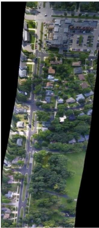
Figure 4.6: Video mosaic result of Perspective video using (a) MoB with P2Prectify, 173 key frames, S_{th}=20 , and non-overlap stitching (c) FB.
