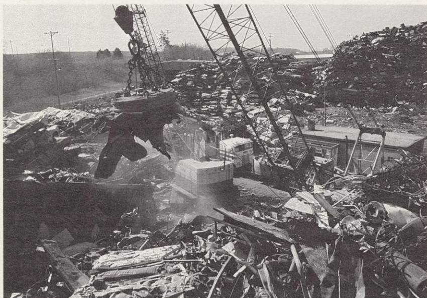
A giant magnet feeds metal into a shredder. Shredders cost anywhere from $400,000 to $4-million.
