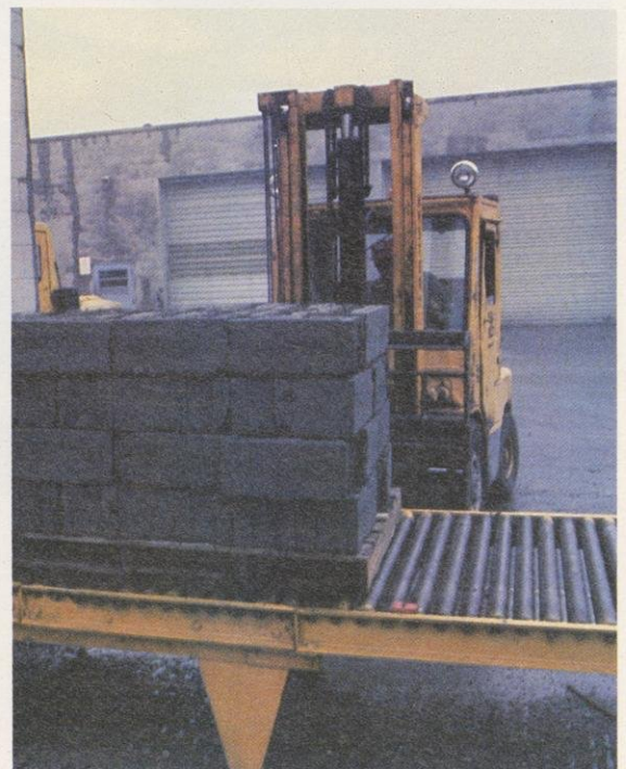
These concrete blocks were made from fly ash by the Wisconsin Electric Power Company. If experiments pan out, they might be used as construction material for a giant Lake Michigan reef to improve fishing. Fly ash is the material collected from smokestacks to prevent air pollution. Together with bottom ash, 1.1-million tons are sent to Wisconsin landfills every year. Many utilities are already marketing fly ash as an ingredient of concrete.
