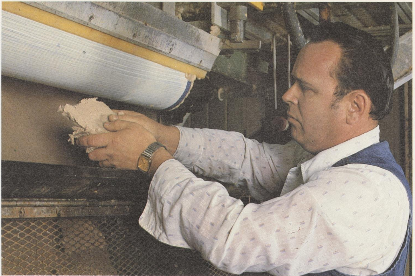
These rollers press the water out of papermill sludge so that it occupies 50% less space in a landfill. Wisconsin Paper Council photo
