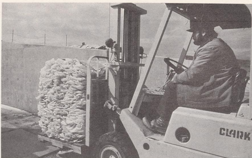
Milk bottles are the largest single source of recycled plastic in Wisconsin. They have to be crushed and baled prior to sale.
