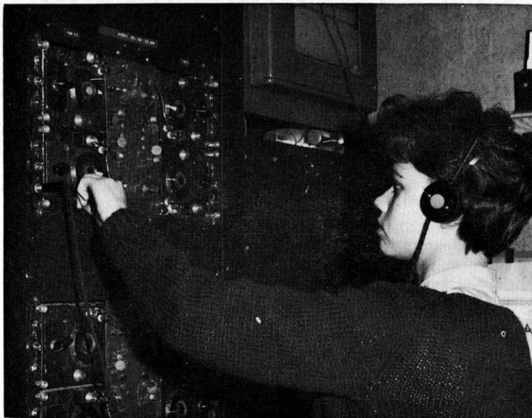
JUST LIKE TUNING IN A RADIO STATION, A RECEIVER IS TUNED IN TO THE PROPER FREQUENCY TO DETECT THE SIGNALS FROM A BARRED OWL LOCATED IN A DENSE OAK WOODS. RECEIVER AT LEFT DETECTS SIGNALS FROM A 100-FOOT TOWER WHILE RECEIVER AT RIGHT DETECTS SIGNALS FROM A 70-FOOT TOWER. DEGREE BEARINGS OBTAINED FROM THE TWO TOWERS PERMIT THE OWL TO BE LOCATED ON A MAP BY TRIANGULATION. PHOTO BY NICHOLLS.
