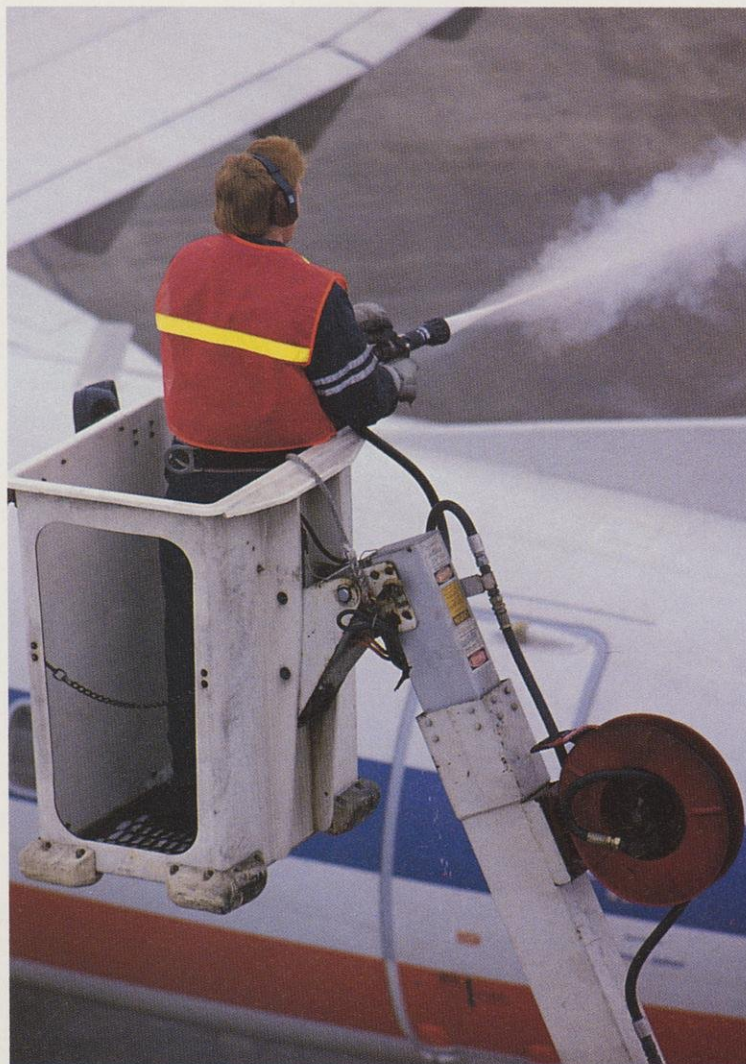
De-icers can be applied September through May in Wisconsin when wings can ice up at higher altitudes.
