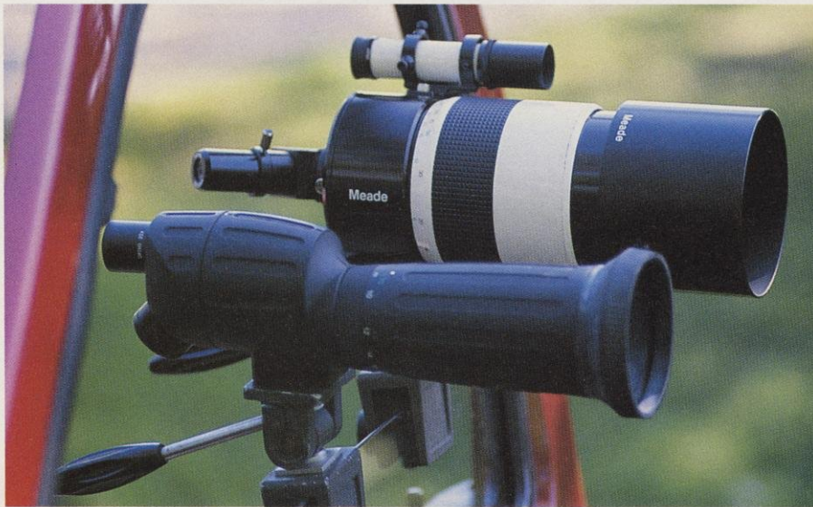
Many spotting scopes can be attached to window mounts or tripods. Scopes make animals appear closer, but they transmit less light than binoculars. Refracting scopes (left) use lenses to bend light rays. Reflective or mirror scope (right) use mirrors. Reflecting scopes are lighter, but more delicate. They are more often by those who want to watch birds and do some star gazing.
