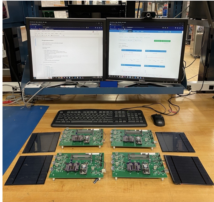
Figure 9.5: Photograph of multiple Pico boards that fit easily on a lab bench.
