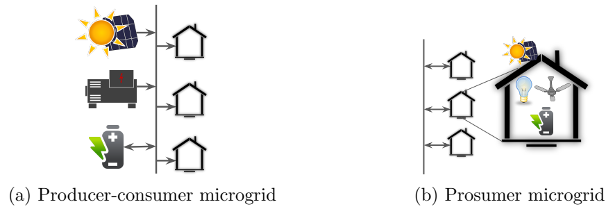
Figure 9.1: A sketch of microgrid architectures
