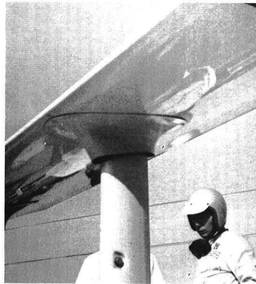
Above: Veteran car owner-designer Jim Hall ponders the prospect of his winged machine getting the best of him. The wing is movable and functions like an airplane flap.
