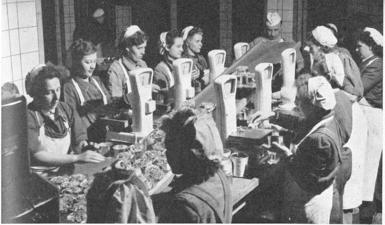
Prior to sealing, meat in each can is checked for correct weight. Five grams are added to guaranteed correct weight.
