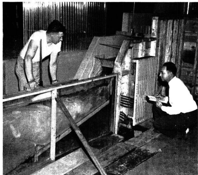
Determining water action from model flume. Professor A. T. Lenz in the foreground.
