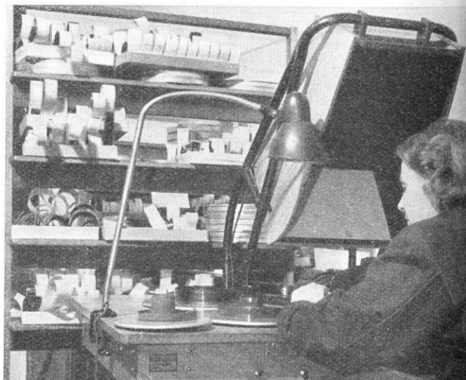
Checking as many as 20 recordings of a single scene, operator watches a short run to select the one which corresponds best to lip movements of the original film.
