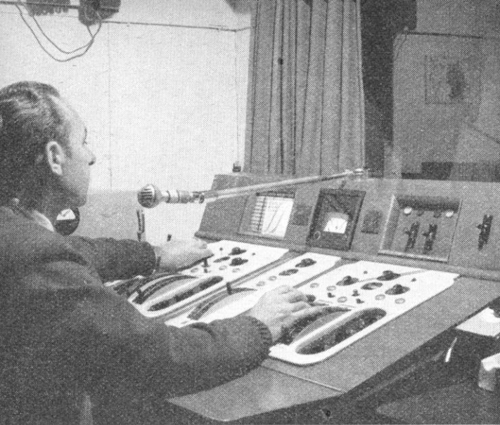
Technician manipulates buttons, switches and dials on "mixing table" to control recording of new voices for synchronization of German in place of original dialogue.
